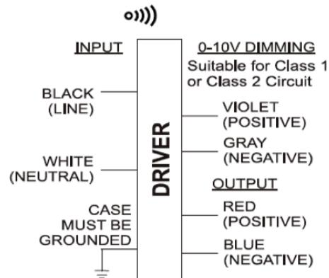
Input and output use lead-wires.
